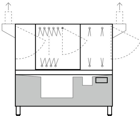
**BASIC MACHINE.** With pump rinse and compact dimensions. In linear configuration or as corner installation. Improves the rinse result and provides a slight increase in machine capacity.
