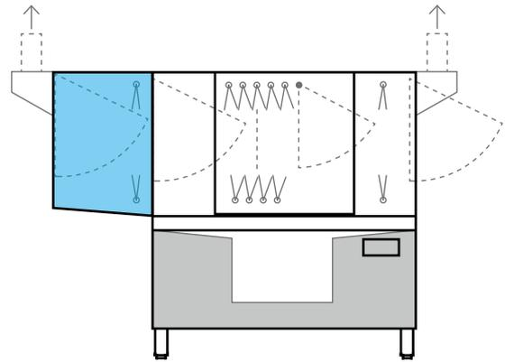
**WITH PRE-CLEANING ZONE.** For increasing the machine capacity with a higher volume of wash items. Optionally available and can be retrofitted later.
