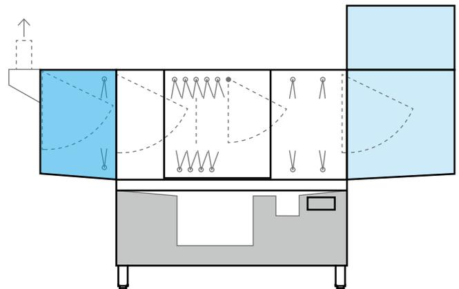
**WITH PRE-CLEANING AND DRYING ZONE.** When the cleaned wash items have to be immediately reusable even at peak times. Both zones are optionally available and can be retrofitted later. Including pump rinse for an improved rinse result.
