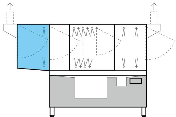
**WITH PRE-CLEANING ZONE.** For increasing the machine capacity with a higher volume of wash items. Optionally available and can be retrofitted later. Including pump rinse for an improved rinse result.
