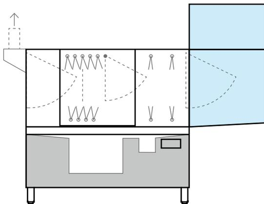
**WITH DRYING ZONE.** This allows the wash items to be used again straight away. Optionally available and can be retrofitted later. Including pump rinse for an improved rinse result.
