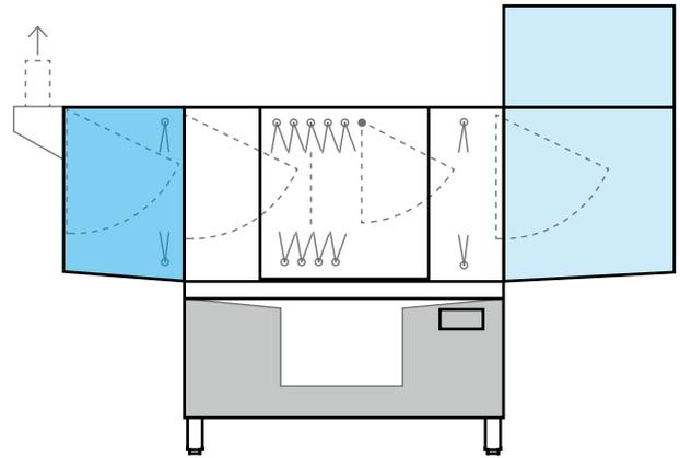
**WITH PRE-CLEANING AND DRYING ZONE.** When the cleaned wash items have to be immediately reusable even at peak times. Both zones are optionally available and can be retrofitted later.
